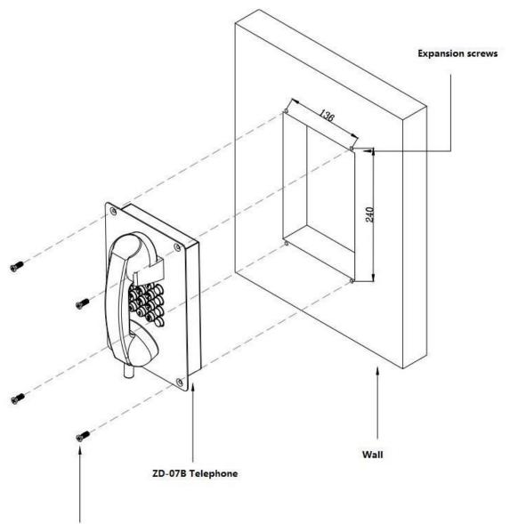
4-M5\*20Cross countersunk head machine screw
